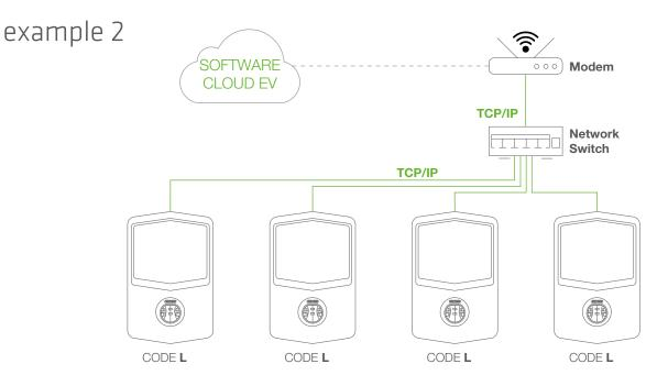
The charging stations are all equipped with Ethernet Kit (version «L»), and are all wired in the centre of the star within a switch. Connectivity takes place through a Router available in the system.
