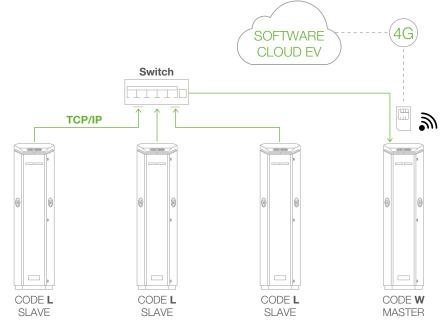
The charging stations are all equipped with Ethernet Kit (version «L») are wired in the center of the star within a Switch. Data is then transferred to THE MASTER station that integrates a Router and the SIM is wired in and out with TCP/IP line and only the last charging station has a 4G SIM that communicates with the backend via OCPP 1.6 JSON protocol.
