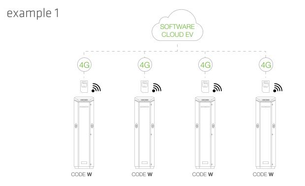
Charging stations are all equipped with Kit Router 4G (version «W») and communicate «Peer To Peer» with the communication backend via OCPP 1.6 JSON protocol.
