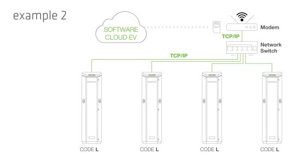
The charging stations are all equipped with Ethernet Kit (version «L»), and are all wired in the centre of the star within a switch. Connectivity takes place through a Router available in the system.
