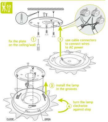
2.2 2nd method: mounting on the wall with the connection to the outlet, using the cable supplied
